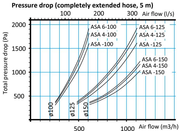
Systems are normally designed for stationary vehicles, but the air flow should be selected higher than stated exhaust gas flow. The system as a whole should be designed for a somewhat higher load than stated by minimum requirements.
