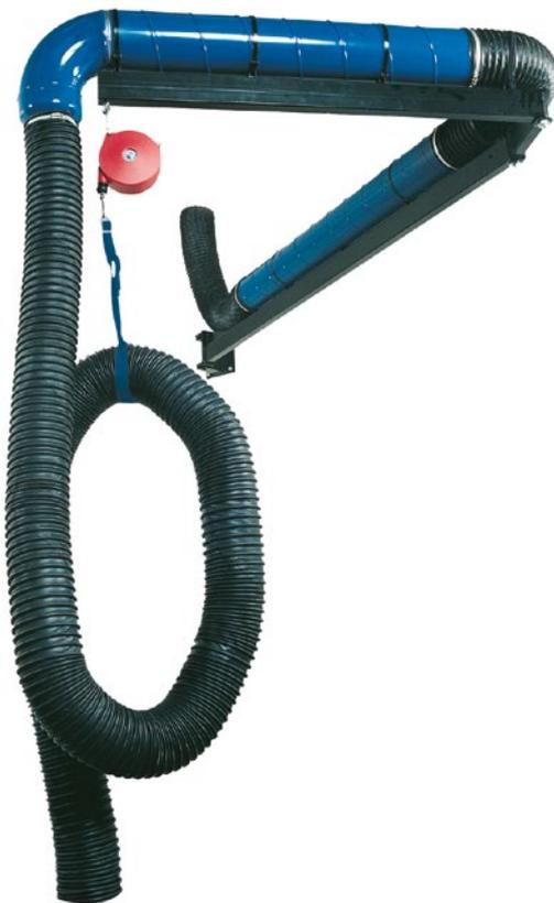
The Fumex balancing block solution, type ASA without pivoting arm, is equipped with hose, balancing block and suspension belt. The extractor is mounted hanging from the ceiling or other high location. For wall mounting, wall bracket ASA V is available.
